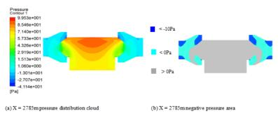
Fig. 5. Pressure distribution contours
