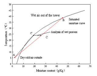
Fig. 2. Plume generation and elimination theory
