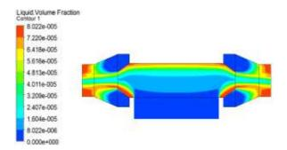
Fig. 8. Liquid water volume fraction distribution cloud of X = 2785 m
